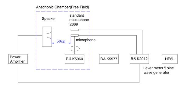
7.3.1 Testing microphone with the standard operating condition.
